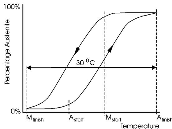
Fig. 1. Transition trajectory for a typical NiTiCu SMA. The phase transition from Martensite to Austenite takes place within 30°C. There is a hysteresis in the transition temperatures between  $M_{finish}$  to  $A_{finish}$  and from  $A_{finish}$  to  $M_{finish}$ .
