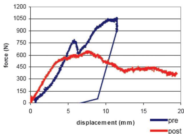
Figure 2. Force/displacement graph in partial VB height PMMA filling.
