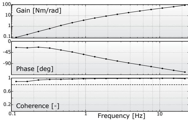
Fig. 10. Bode plot of the minimal impedance measurements, with impedance  $H_{img} = T_{act}/\theta_{jnt}$ . For these measurements, the reference torque  $T_{ref}$  is 0 Nm, while the angular position  $\theta_{jnt}$  was perturbed by a 0.1-25 Hz multi-sine with two times the standard deviation equal to 0.1 rad.
