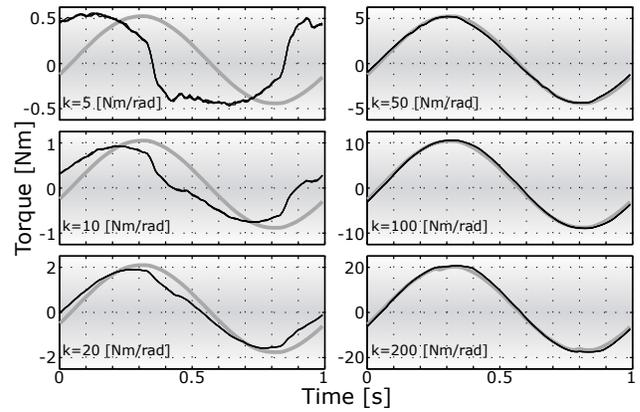
Fig. 12. Time plots of virtual springs. The external motor maintained a 1 Hz sine with a 0.1 rad amplitude on the angular position  $\theta_{jnt}$ , while the virtual spring stiffness was increased from 5 to 200 Nm/rad. (Note the real spring stiffness of 88 Nm/rad.) The gray lines are the measured joint angles  $\theta_{jnt}$  multiplied by the virtual spring stiffness, resulting in the desired torque signal  $T_{ref}$ . The recorded actuator torques and plotted in black.
