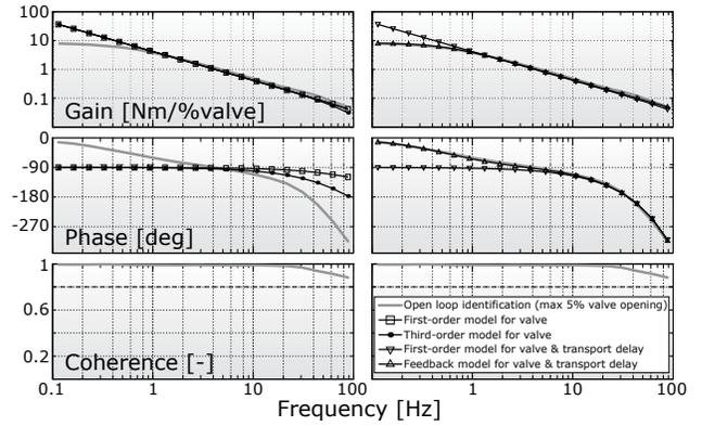
Fig. 7. Bode plot of the open-loop identification of the complete actuator  $H_{act,ol} = T_{act}/u$ . The open-loop results were fitted with actuator models  $H_{act,ol1-4}$  consisting of the valve, tube, piston and spring components.  $H_{act,ol1}$ : line with open squares,  $H_{act,ol2}$ : line with closed circles,  $H_{act,ol3}$ : line with downwards pointing triangles,  $H_{act,ol4}$ : line with triangles pointing up.  $H_{act,ol4}$  clearly results in the best fit.
