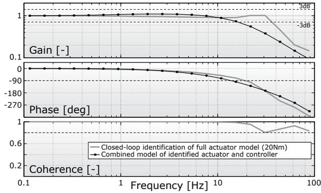
Fig. 8. Bode plot of the closed-loop frequency response function  $H_{sys,cl} = T_{act}/T_{ref}$  for the 20 Nm multi-sine reference torque (the gray line). The best fitting actuator model ( $H_{act,ol4}$ ) was combined with the system model  $H_{sys}$ . With the closed-loop control gains, the fit was far from perfect (line with filled circles).
