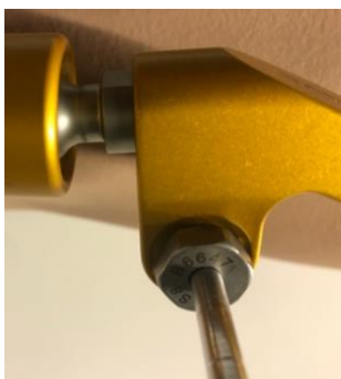
Figure 27 Place Half-pin locking bolt over the Half-pin
