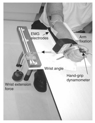
**FIGURE 2.** Test position of the arm in the laboratory setup. The angle of the wrist can be securely positioned and reproduced. The arm is stabilized at the wrist. The wrist extension force is applied by a mass, which is attached via a cable to a strap around the palm of the hand at an angle of 90° (by adjusting the position on the rails).
