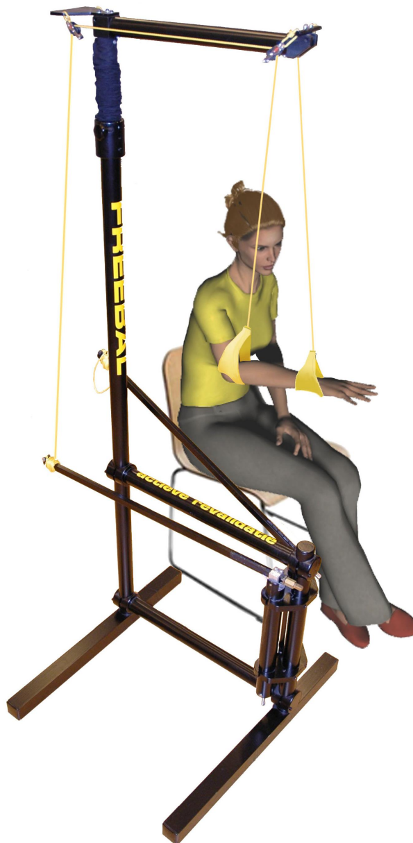
Fig. 1. Freebal gravity compensation system, which generates the compensation force with an almost inertia-free ideal-spring mechanism (see Fig. 2). The wrist and elbow of subjects are hung in the two slings supports of the Freebal. For graphical reasons, the Freebal is here shown with the lowered overhanging beam instead of the normal 3.5 m above ground level.
